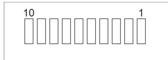
**AT/ATX Mode Selection Header**
