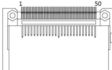
**Mini PCIe: Mini PCIE connect**
