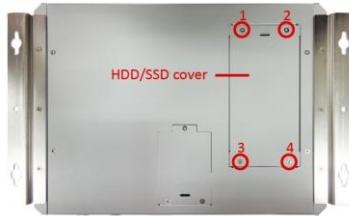
2. Take off the cover. The cover is used to hold a 2.5" SATA HDD/SSD.
