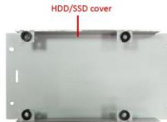
3. There are 4 screws in the accessory packet. Slide the 2.5" SATA HDD/SSD into the HDD/SSD cover, align the mounting holes and fasten the screws
