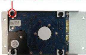
4. Connect SATA power cable and SATA signal cable. Make sure the cables are well connected. Fastener HDD/SSD cover screws.
