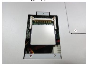
3. Make sure CF-SATA card is completely seated. Fastener CF-SATA card cover screws.
