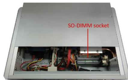
3. Insert the module into the socket.
