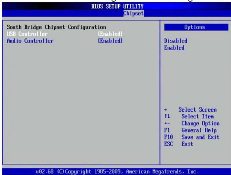
**USB Controller:** this field is used to enable or disable the Enhanced Host Controller Interface.
